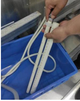
Rinse the sprinkler pipe and core rod
